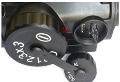
Micro HDMI line HDMI interface of the machine, you can output high-definition video. As shown in figure (4) when high-definition video output, internal display automatically shut down.
